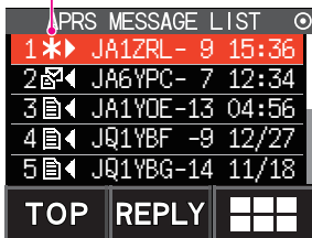
APRS MESSAGE LIST screen (display when an acknowledgment is received)
